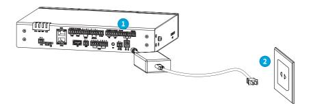
**Step 1** Connect the power adapter to the EzLogger.
